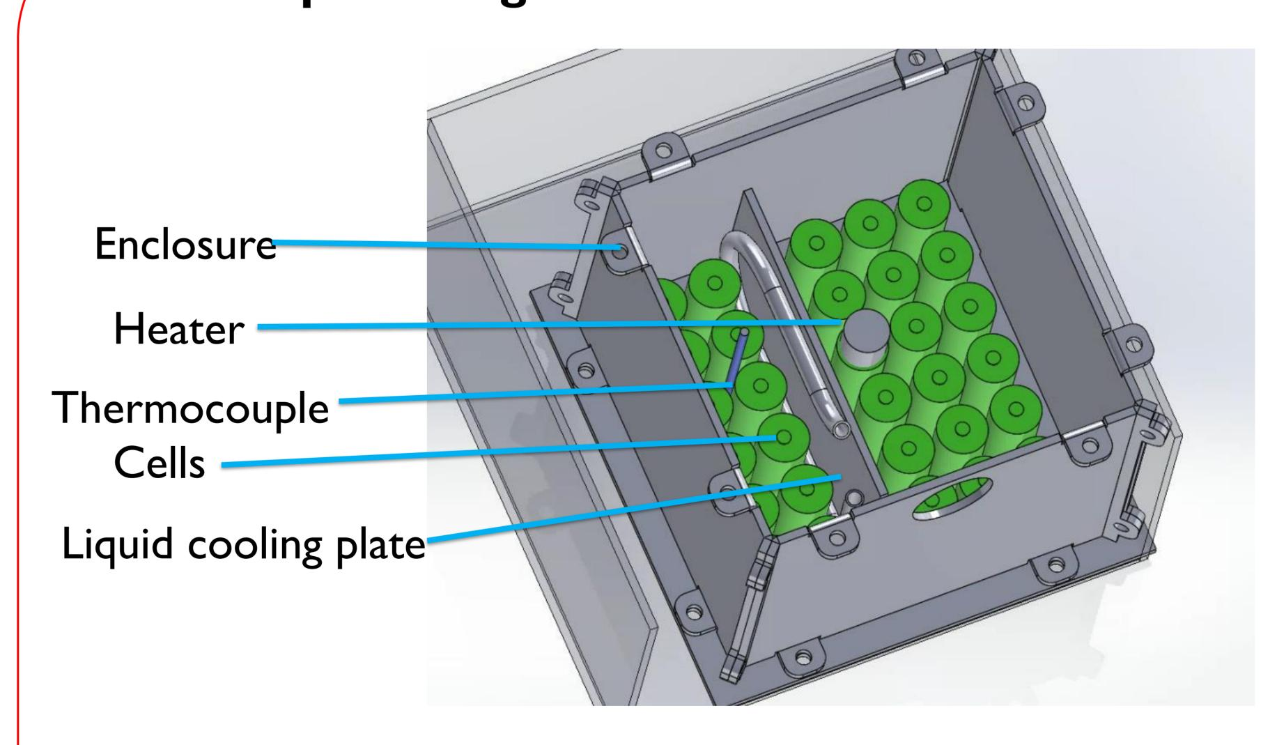
A rig to conduct low power tests and validate the COMSOL model is under development. Designed to mimic an accumulator. This will ensure the conduction, convection and radiation mechanisms are functioning correctly and the rig can be used for final destructive testing.
